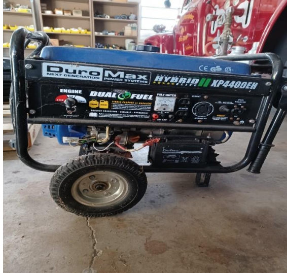
Dual Fuel Generator
