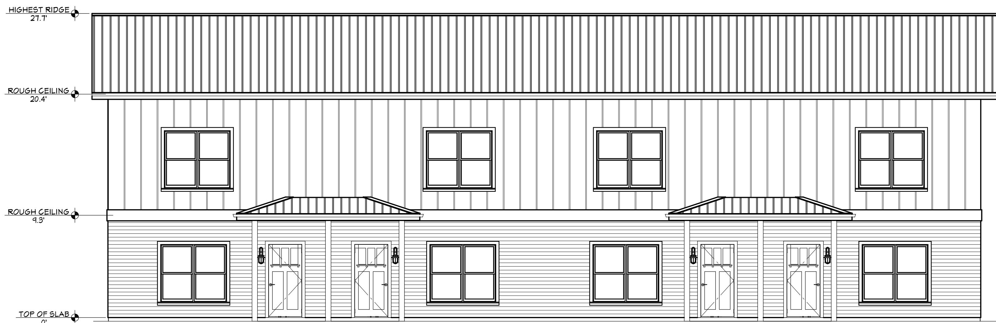
FRONT ELEVATION SCALE: 3/16"=1'
